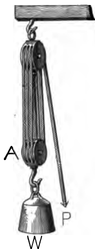
FIG. 172. — An effective arrangement of pulleys known as block and tackle.
